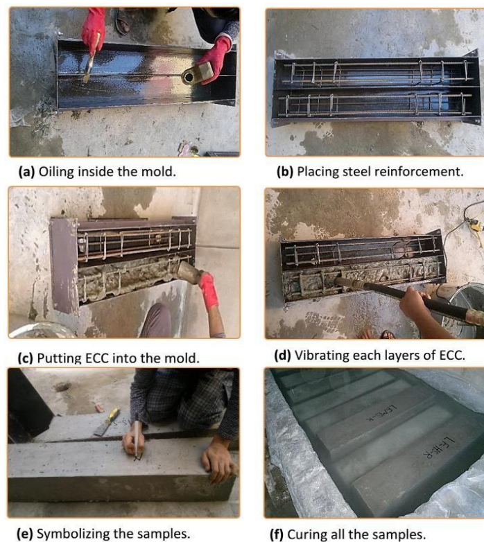
FIGURE 4. Casting and curing steps
