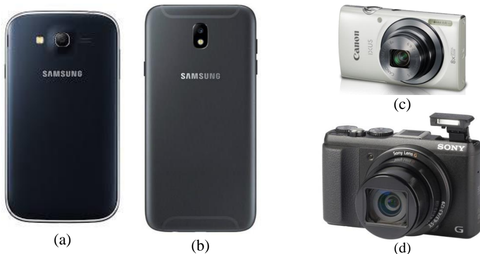
FIGURE 2. used mobile phones (a) Samsung smartphone model GT-I9060I resolution 5 MP (b) Samsung smartphone J730F Galaxy 13 MP (c) Canon compact camera IXUS160 resolution 20 MP (d) Sony Compact Camera HX60V resolution 20.4 MP.
