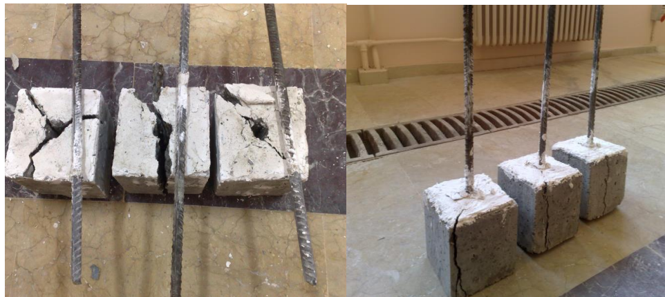
FIGURE 6. Typical failure patterns of concretes a) without fiberreinforcement and b) withfiber reinforcement.
