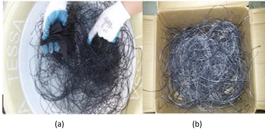
FIGURE 1. A- Recycled steel wires a-before cleaning , b- after cleaning.
