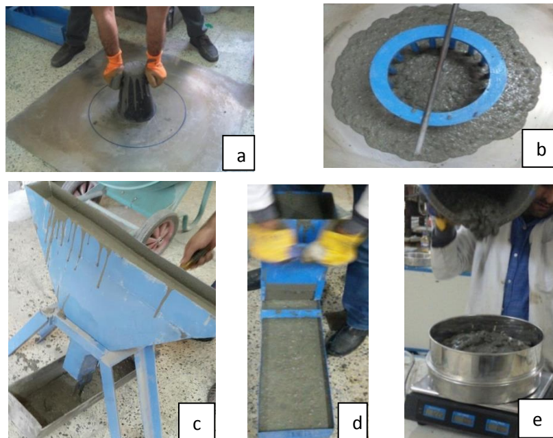
FIGURE 3. Rheological properties tests: (a) slump flow, (b) j-ring, (c)V-funnel, (d) L-box, d-Segregation resistance
