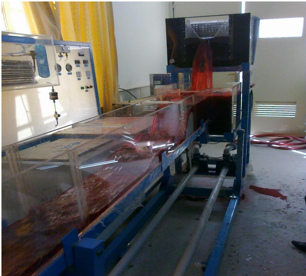
FIGURE 2. General view of the recirculation rectangular channel
