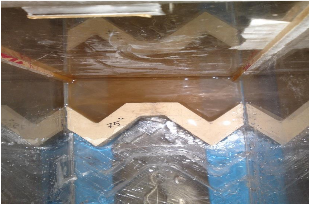
FIGURE 3. One of the W baffle models at angle 75°
