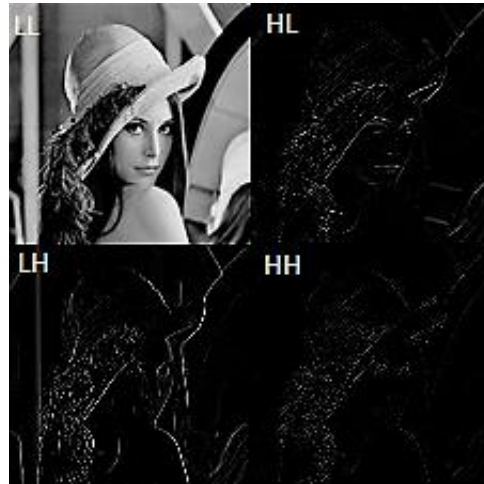
FIGURE 4. 2D-DWT transform on face image
