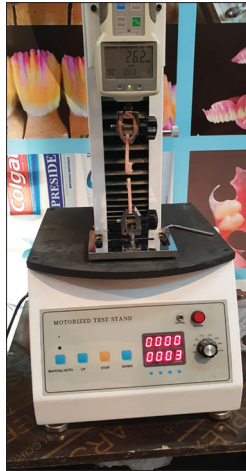
Figure 8: SBS by motorized testing machine
