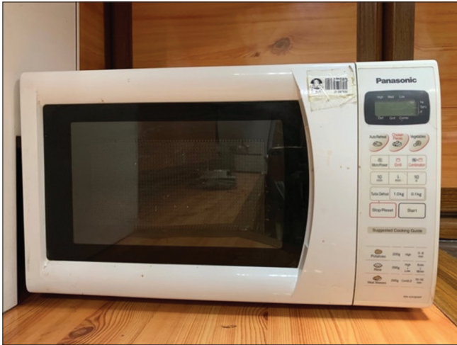
Figure 3: Domestic microwave for polymerizing PMMA microwave cured samples and soft liner
