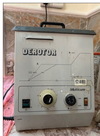
Figure 2: Water bath for polymerizing PMMA water bath cured samples and soft liner
