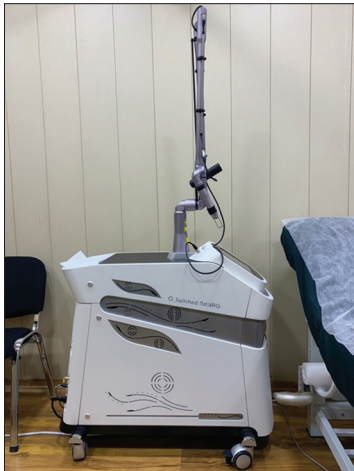
Figure 4: Q switched Nd:YAG device used for PMMA surface treatment
