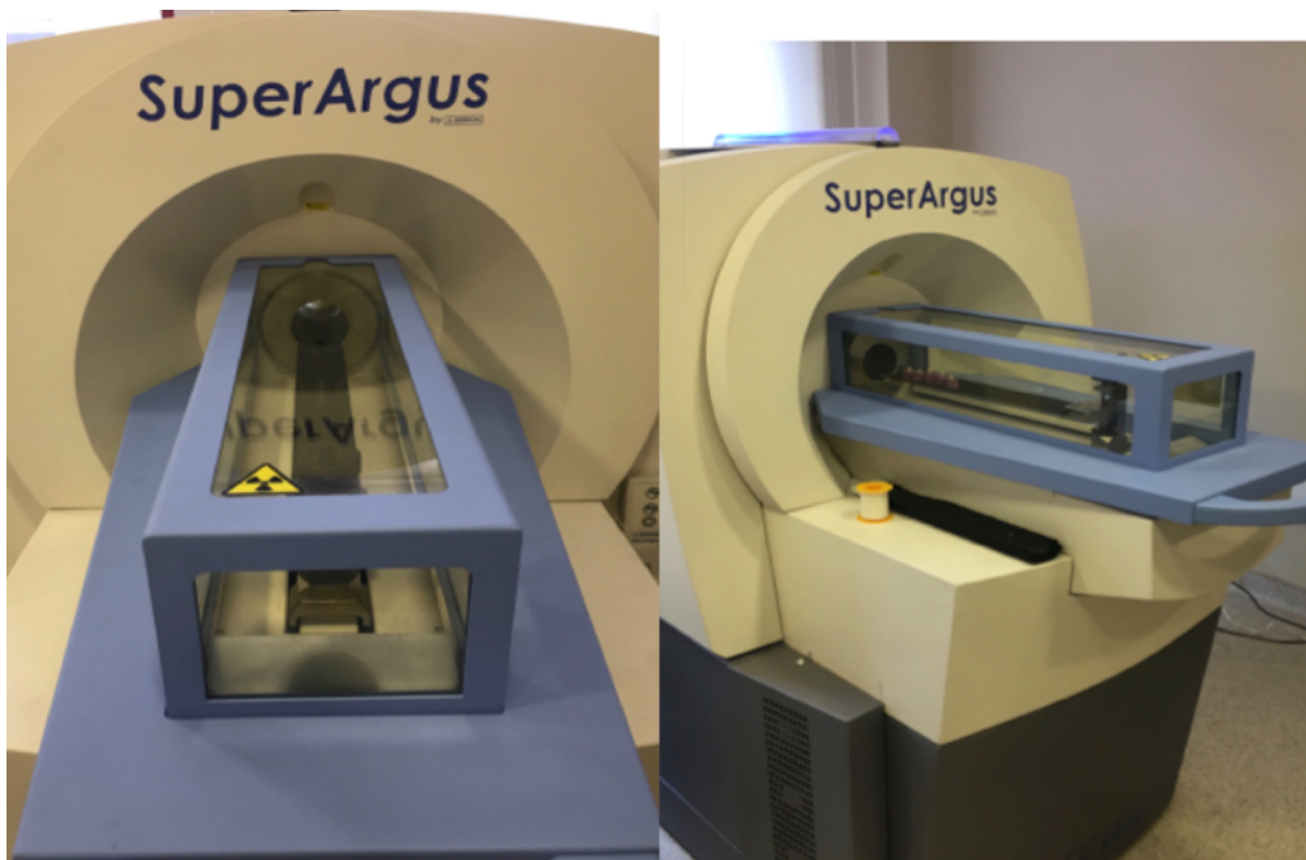
Figure 2: Sedecal/ Super Argus micro-tomography machine.
