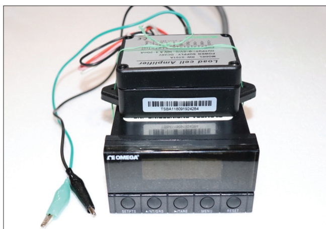
Figure 3: Connection of electric clamp, amplifier, and digital output reader
